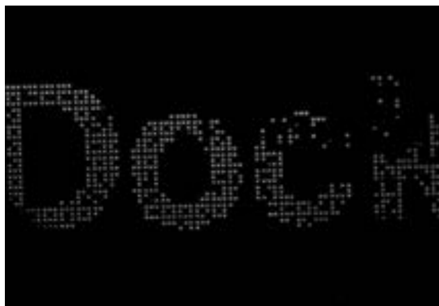
Figure 2. An implementation of spatial ECL ( \text{Ru}(\text{bpy})_3^{2+} based) on the (CMOS1) dock, with each lighted site stimulated by the application of a voltage to a microelectrode (global counter electrode).
