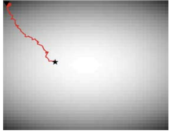
Figure 4: An axis parallel hyper ellipsoid gradient was presented to a swarm executing FSTaxis algorithm. The grayscale shows the gradient value and the goal is the darkest area; the star symbol represents the starting point and the inverted triangle marks where the swarm converged.
