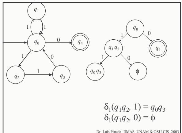
$$\begin{aligned}\delta_1(q_1q_2, 1) &= q_0q_3 \\ \delta_1(q_1q_2, 0) &= \phi\end{aligned}$$
